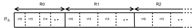
Fig. 2. Resolution scalable bitstream structure. R_0, R_1, \dots denote the different resolutions, t_{16}, t_{15}, \dots the different bitplanes. This bitstream corresponds to the coding of one block B_k .
