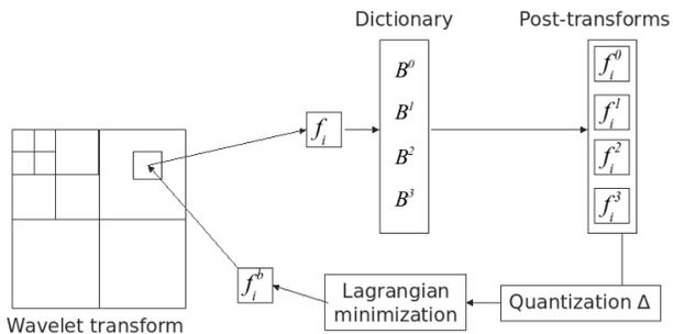
Fig. 1. The post-transform scheme.
