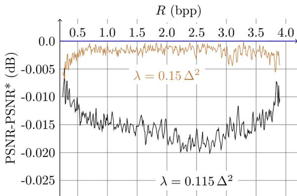
**Fig. 6.** Losses in PSNR using different formulas to compute the Lagrangian multiplier compared to the best achievable PSNR. These are mean results on six Earth observation images.
