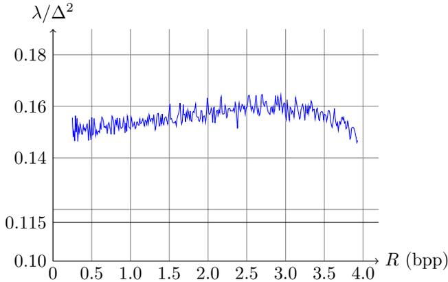
**Fig. 5.** Mean ratio between the optimal Lagrangian multipliers  $\lambda$  and the square of the quantizer steps  $\Delta^2$  on six Earth observation images. This ratio is compared to the theoretical value 0.115 on a wide range of compression bit rates.
