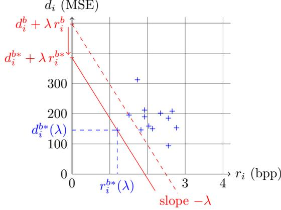
**Fig. 2.** Graphical interpretation of the best basis selection process on one block. Each cross corresponds to the rate-distortion point  $(r_i^b, d_i^b)$  of the quantized representation of  $f_i^b$ . The best basis for the given slope  $-\lambda$  is found by minimizing the quantity  $d_i^b + \lambda r_i^b$ . This quantity can be read at the intersection of the line of slope  $-\lambda$  with the ordinate axis.
