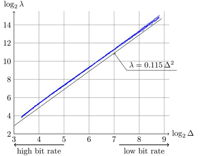
**Fig. 4.** Optimal Lagrangian multipliers  $\lambda$  computed on six Earth observation images compared to the theoretical curve  $\lambda = 0.115 \Delta^2$ .
