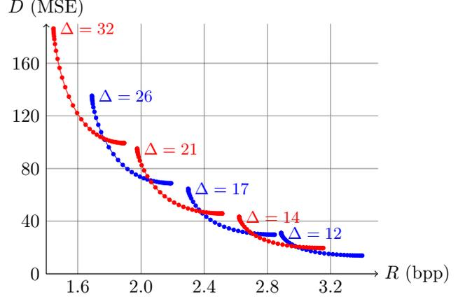
**Fig. 3.** Rate-distortion curves computed on a 12-bit depth image. Each curve is obtained with a fixed quantization step  $\Delta$  and with Lagrangian multipliers  $\lambda$  ranging from 1 to 5000. Each dot corresponds to a value of  $\lambda$ .
