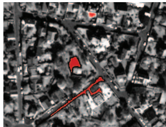
Fig. 3. Segmentation example: from three different seeds. The fast marching algorithm generates three different areas.
