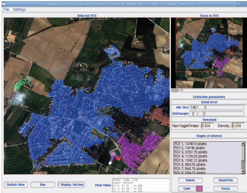
Fig. 2. Automatic urban area extraction using texture features
