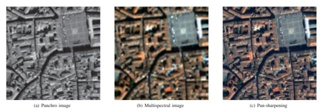
Fig. 6. Pan-sharpening example: high resolution of the panchromatic image is introduced in the multispectral image to obtain a multispectral high resolution image.
